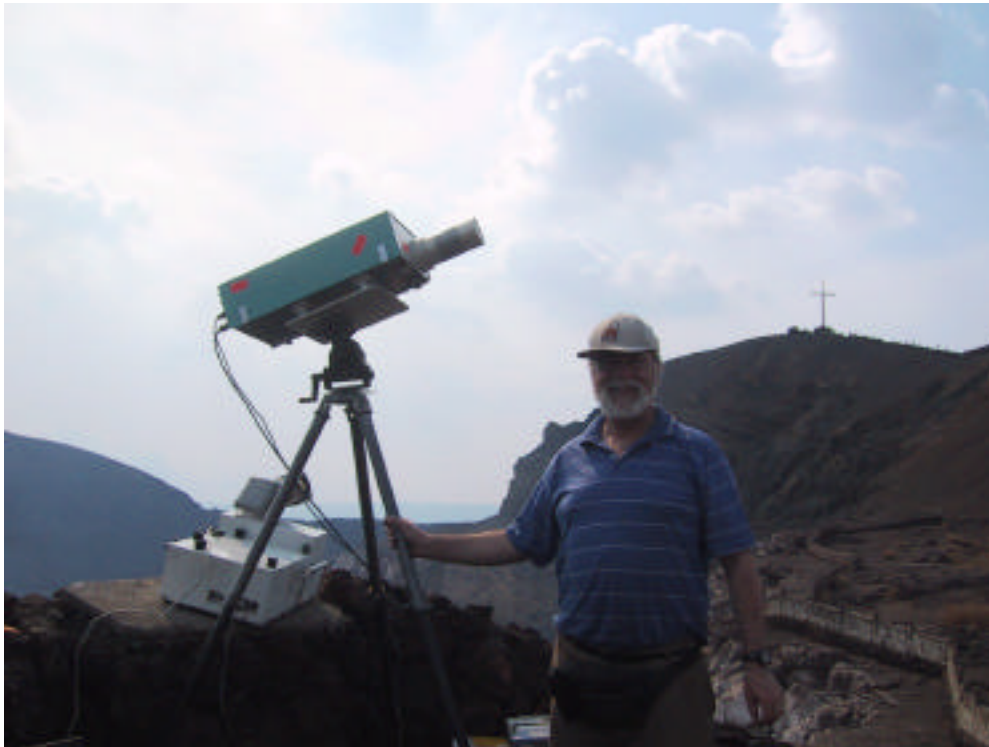
Upper Photo: Dr. Bill Morrow, who is President of Resonance Ltd. of Barrie, Ontario, working at Masaya volcano, Nicaragua, during the 8th Field Workshop on Volcanic Gases. Bill is making measurements of sulfur dioxide with a COSPEC (blue instrument) and of carbon dioxide with a GASPEC (white instrument).
